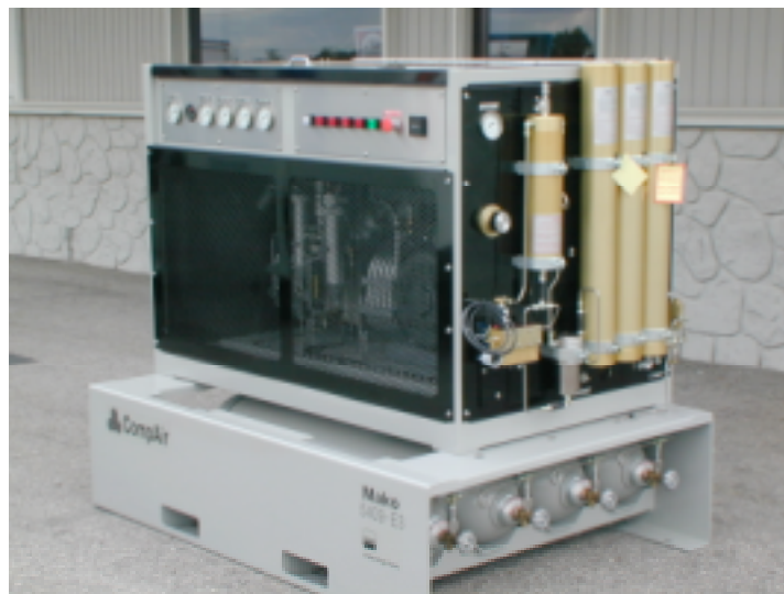
Illustrated: A typical Nitrogen Compressor capable of pressurizing the gas to approximately 2000 PSI ( 140 bar)
