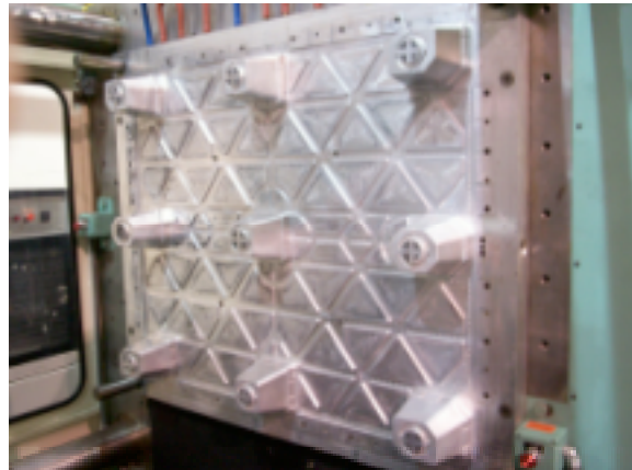
Illustrated: Female and male halves of a typical aluminum mold for making a stackable structural foam plastic pallet.
