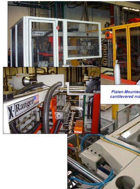
Illustrated: Typical side entry type robot as manufactured by Ranger
