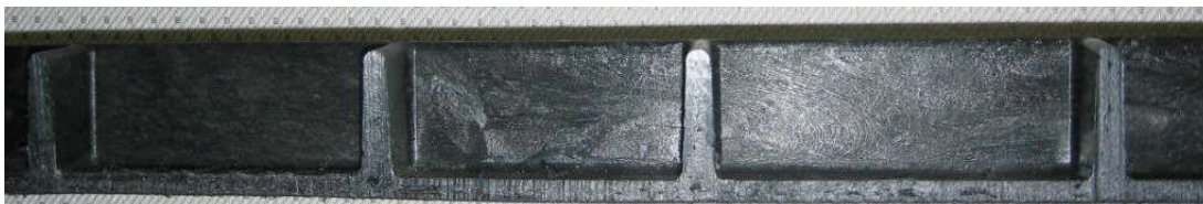
Illustrated: Section of a structural foam plastic pallet showing freedom of form, strength of ribs, and the integral skin, cellular core.
