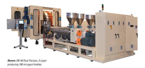
Wilmington's Small Bottle Series Rotary Blow Molding Machines are designed for the production of small/medium single serve drink bottles and foodstuffs, from 80 ml to 12 oz. at rates of 240 to 1,200 bottles per minute. Single or dual parison, 1-6 layers.
